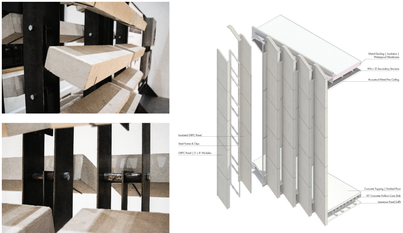
Figure 4. Final fabrication details of Timothy Struempth + Mitchell Culbertson in fall 2018 (right) compared with the final detailed axonometric of Timothy Struempth in spring 2019. Image credit: Genevieve Baudoin and Timothy Struempth.
